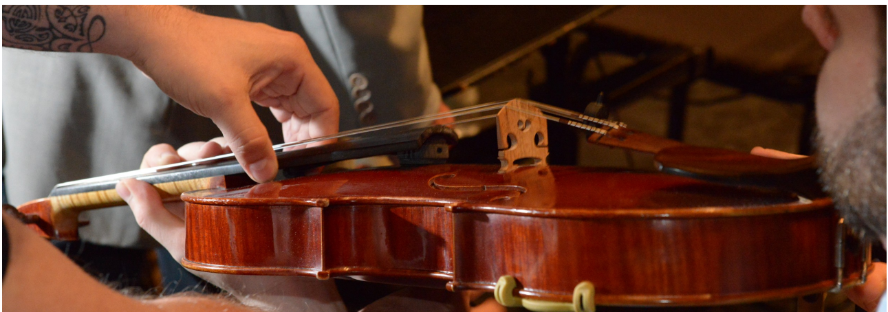
A REMIC microphone is mounted on a violin.
